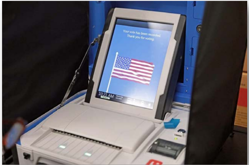
Precinct Scanner with Privacy Screen
